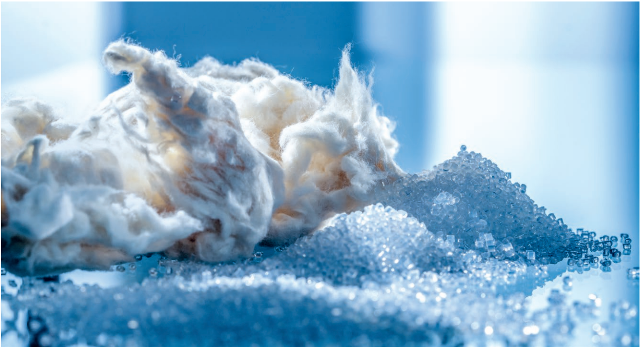
Banknote substrate is made of either cotton or polymer, or a combination of both.
